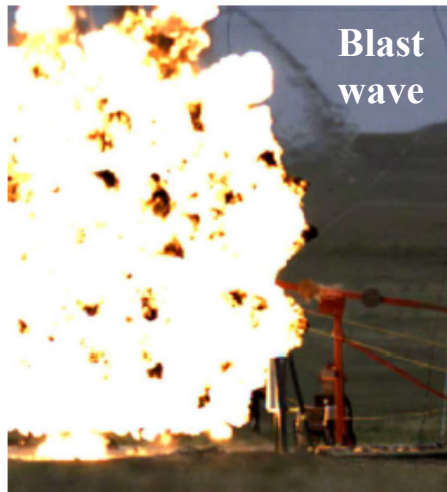
Strong blast wave ahead of fireball from a homogeneous C-4 detonation
