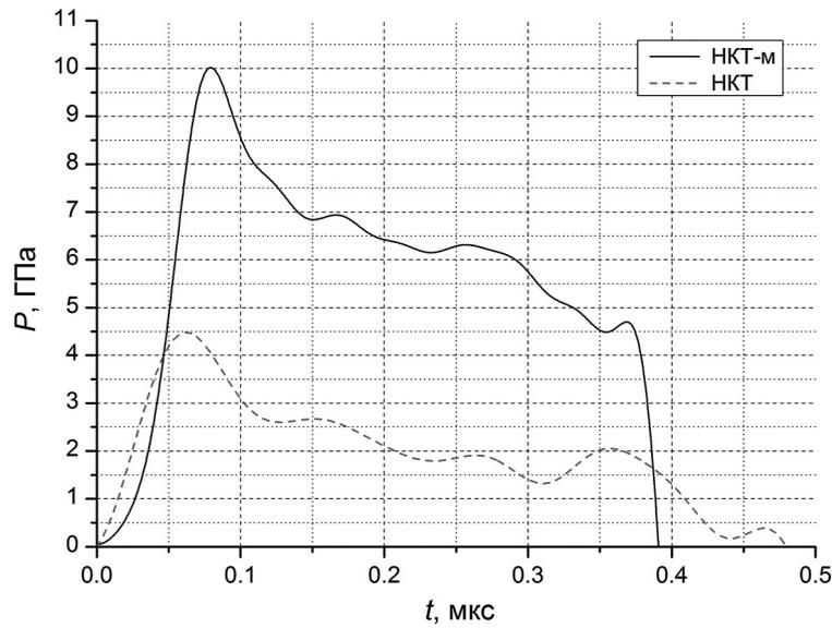
Fig. 3. Pressure profiles on explosion front in pressed samples made of NCP and NCP-m HE
