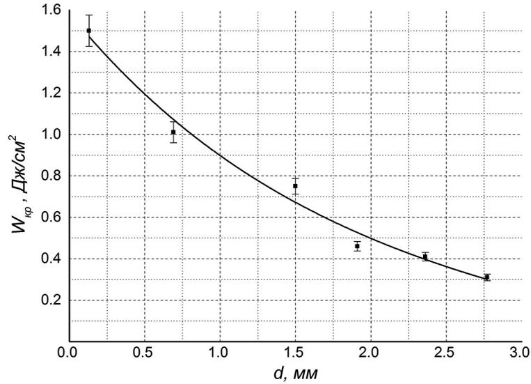
Fig. 2. Threshold energy density,  $W_{cr}$ , of initiating the NCP-m samples vs. light spot diameter,  $d$
