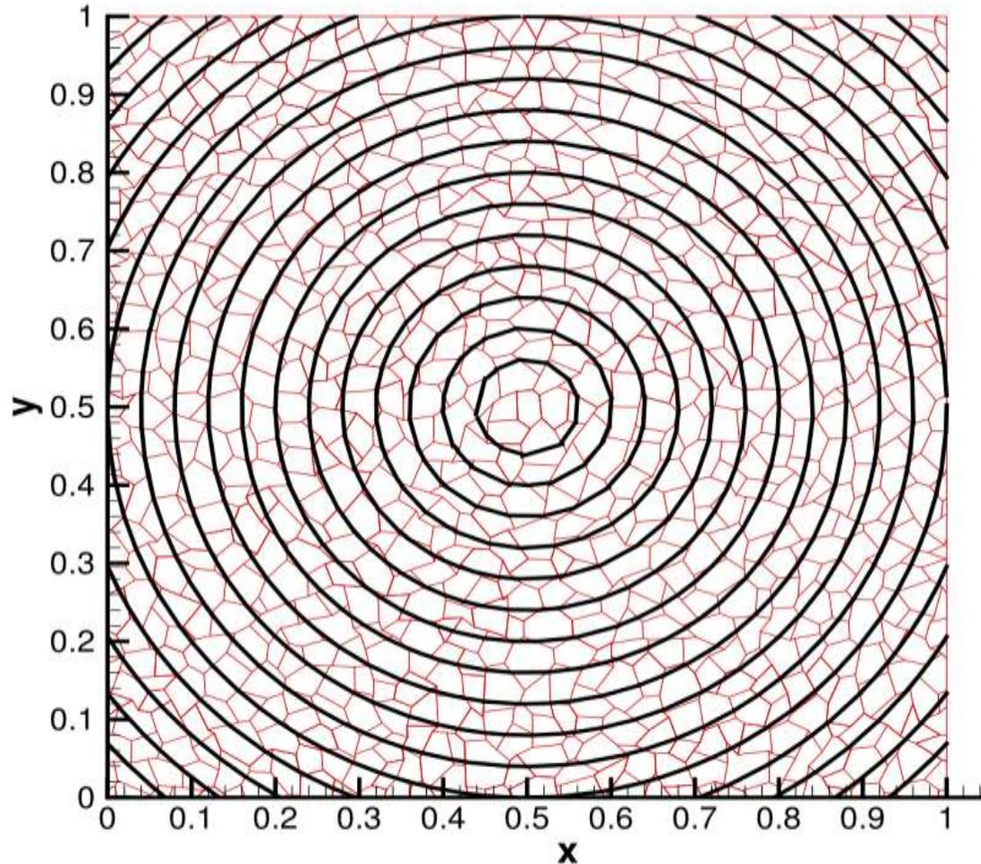
It can be seen that the SVoF algorithm is accurate and effective for reconstruction of three-material cells.
