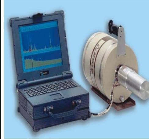
Semiconductor (HPGe) spectrometers (Canberra, ORTEC)
