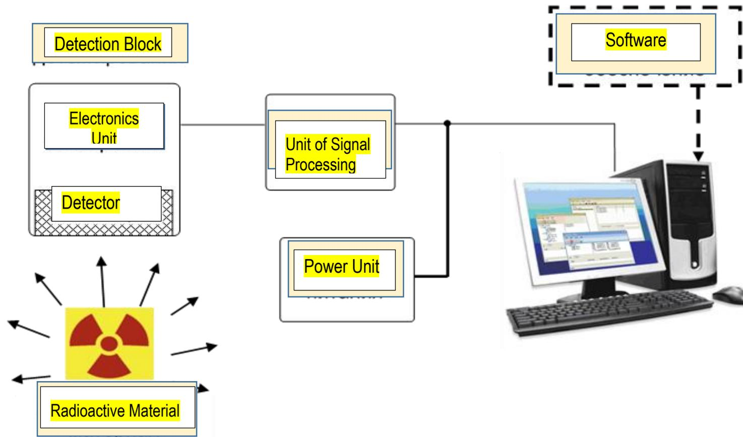
Fig. 1 – Block-diagram of nuclear radiation registration.
