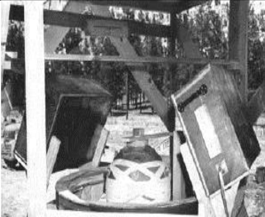
Fig.7. Implosion system and registration blocs.
