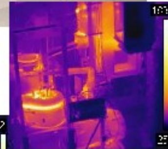
Thermal images of loop containing hot salt
