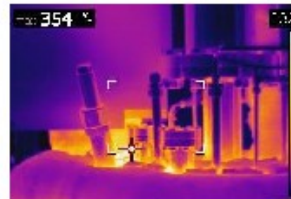
Thermal images of loop containing hot salt
