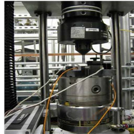
MTS electro-magnetic load frame
