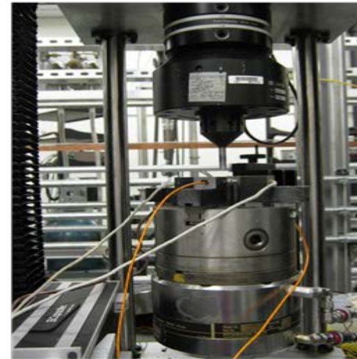
MTS electro-magnetic load frame
