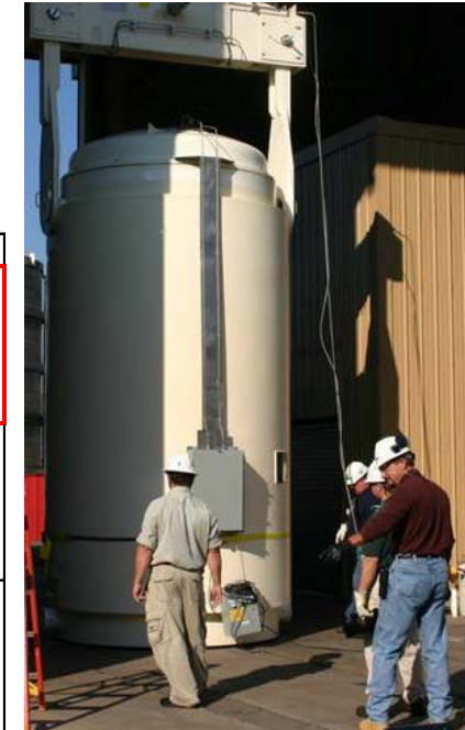
TN-32B cask for the High Burnup Spent Fuel Data Project
