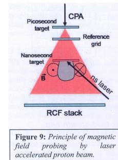
Figure 9: Principle of magnetic field probing by laser accelerated proton beam.
