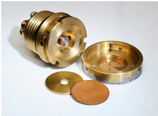
Disassembled current collector head
