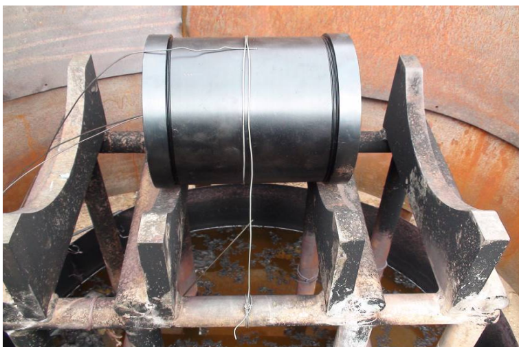
Fig.6 Photograph of fast cook-off test for explosive component
