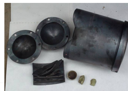
Fig.12 Photographs of scrap in fast cook-off test for PBX-6 explosive component
