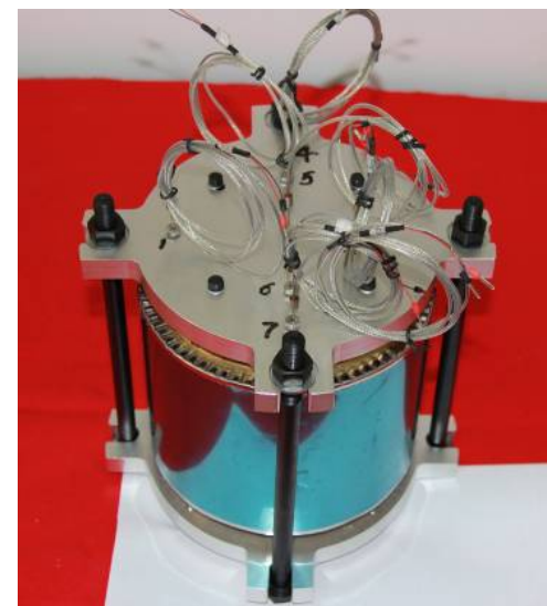
Fig.7 Photograph of slow cook-off test setup of encased thermocouples and explosive components
