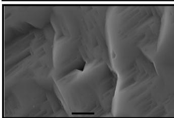
Figure 6: Shocked quartz has multiple planes of deformation. Here, at least 3 planes are present. Bar for scale is 2 microns.
