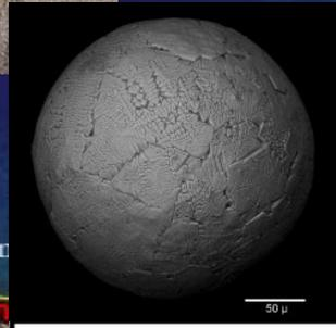
Figure 3: Magnetite spherule with distinctive quench texture indicative of rapid cooling. A bimodal distribution at 85 and 125 microns suggests multiple craters. Bar for scale is 50 microns.
