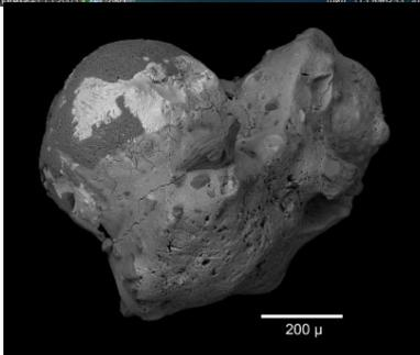
Figure 5: Magnetite spherule (upper left) melting out of a siderite grain.
