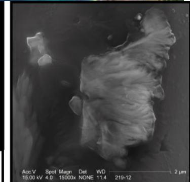
Figure 4: Cr-Fe-Ni splash found on a grain from VC1. Splashes are common on many samples. This one has a dendritic texture.
