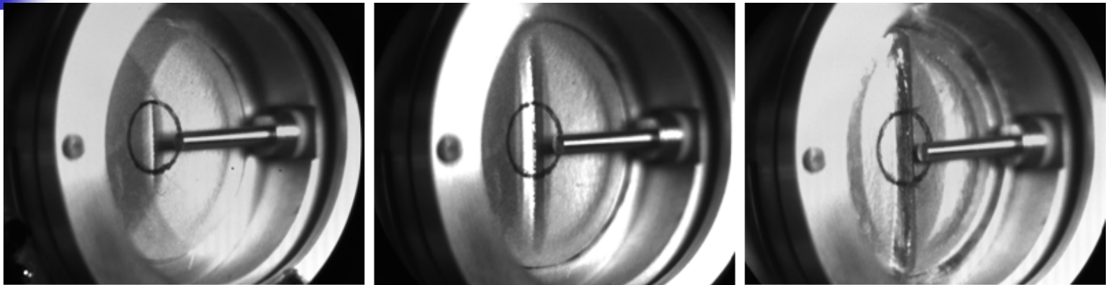
Surface movement on W flyer : regular reflection configuration
