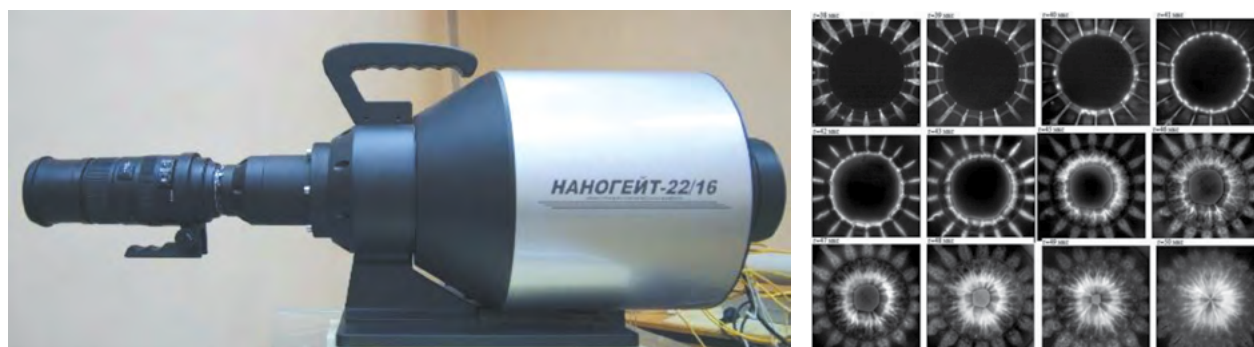
Fig. 1. On the left – camera NANOGATE 22/16, on the right – registration of the detonation process, 12 frames from 16
