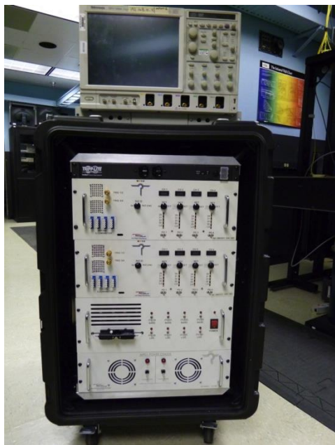
MPDV Prototype 32-Probe System 1x, 2x, 4x, 8x or 16x multiplexing (circa August 2011)
